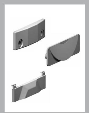
ASSA ABLOY's wide range of wedges work in conjunction with the window fasteners to ensure a tight seal between the window sash and the window frame. All conventional window fasteners require a wedge to be fitted to the window frame, providing a surface for the tongue of the window fastener to compress and seal for a watertight window.
